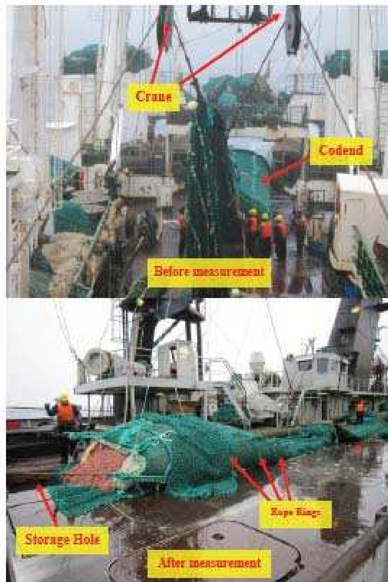
Figure 2. Photos of the deck operations with indications of the codend measurement method
