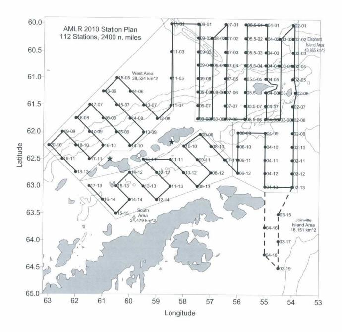
Figure 1. AMLR 2010 station plan. Black dots indicate station locations; heavy lines indicate transects between stations; thin lines outline stratum; stars indicate locations of Cape Shirreff and Copacabana field camps; depth contours are 1000, 2000, and 3000 m. Surveys will be conducted in the following order: West Area, then Elephant Island Area, then Joinville Island Area, then stations in northwest Weddell Sea (if ice conditions permit), then South Area.
