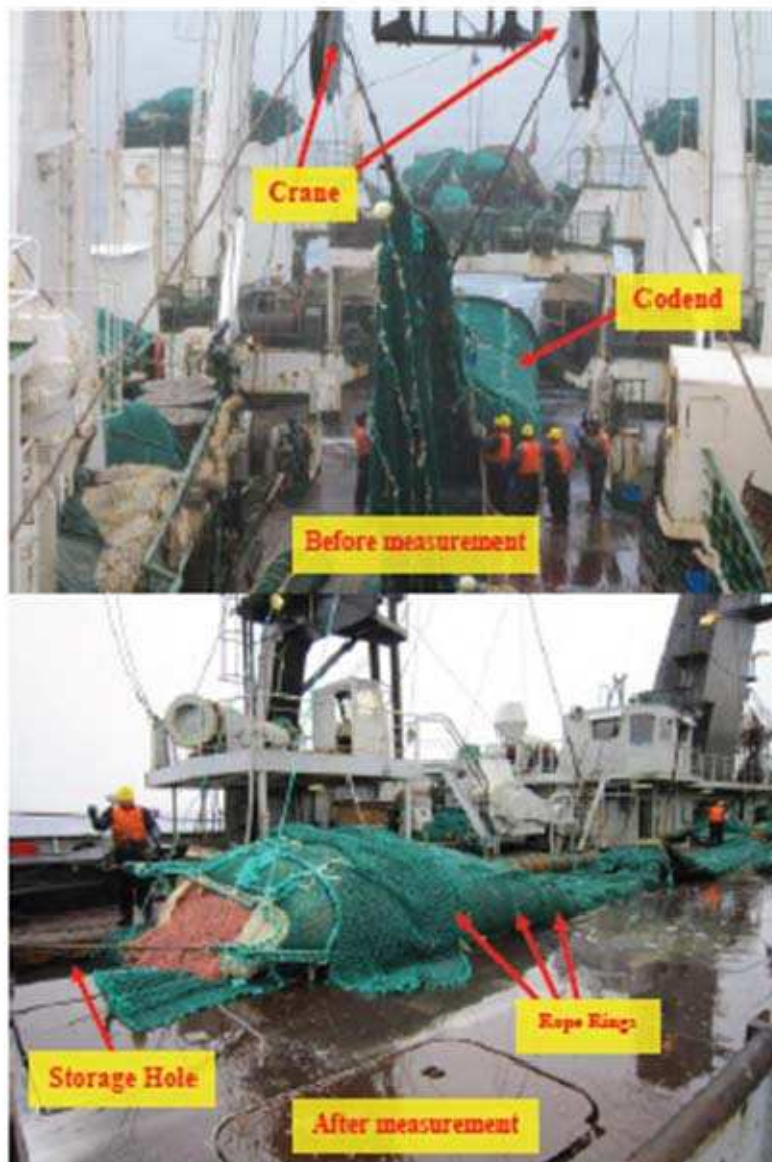
Fig.2 Photos of the landing operations with indications of the codend measurement method
